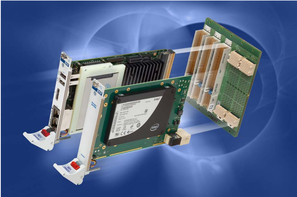
CompactPCI® PlusIO CPU Card as System Controller in a Hybrid System
