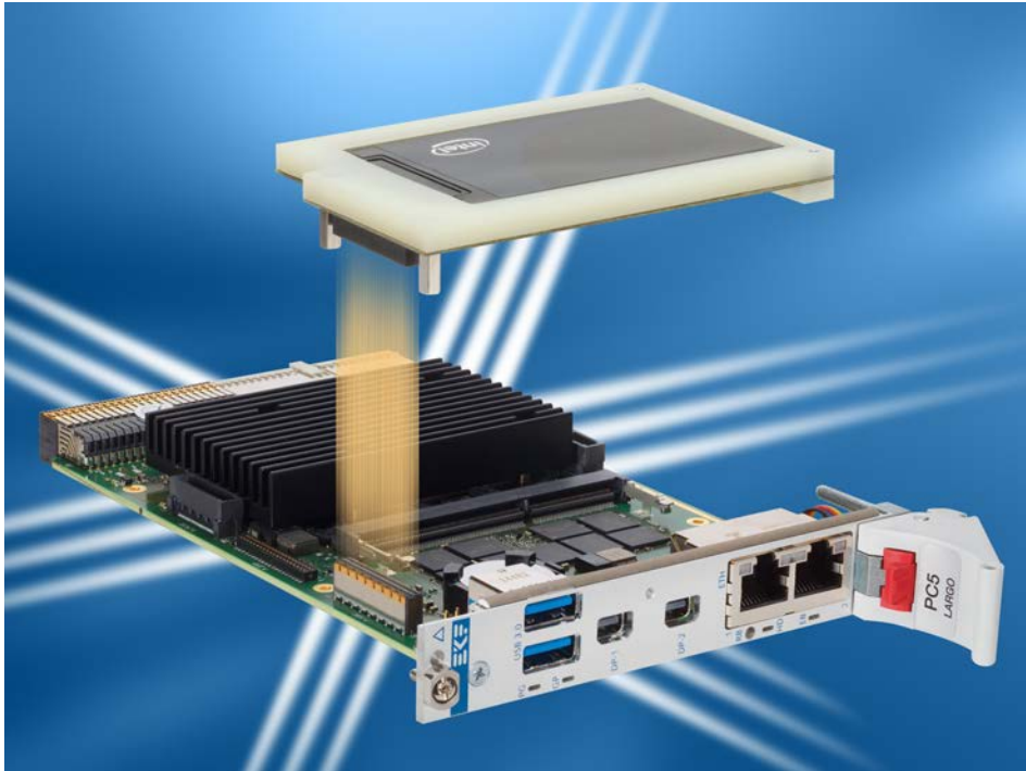
Sample Low Profile Mezzanine Module 4HP Assembly
