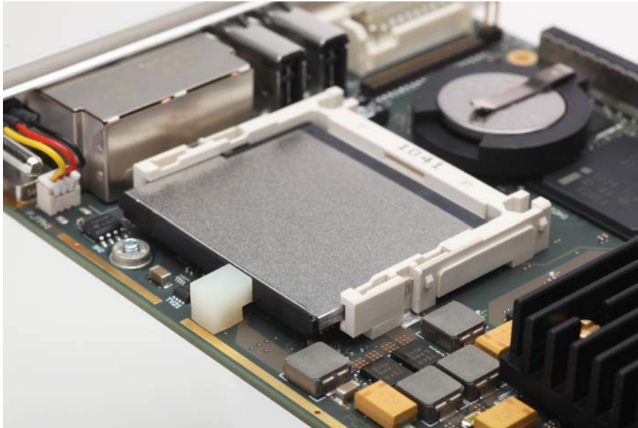
CFast™ Card Fixation w. Mounting Block
